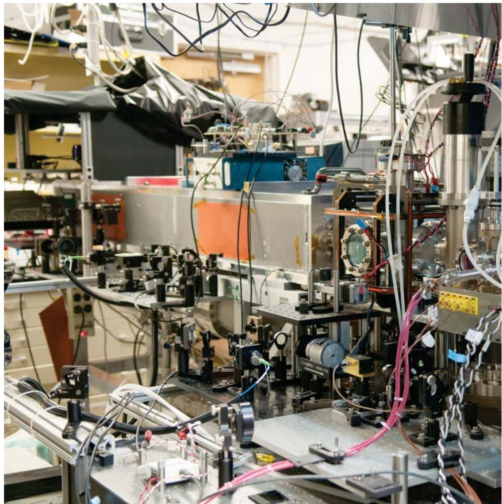
**LITHIUM-7 AS A TEST CASE** was successfully purified by magnetically activated and guided isotope separation with the lab setup shown here. The oven for heating lithium is sitting on the red lab jack to the right. Circular view ports were used for shining lasers to optically pump the isotopes. Inside the rectangular box are the magnetic guides.
