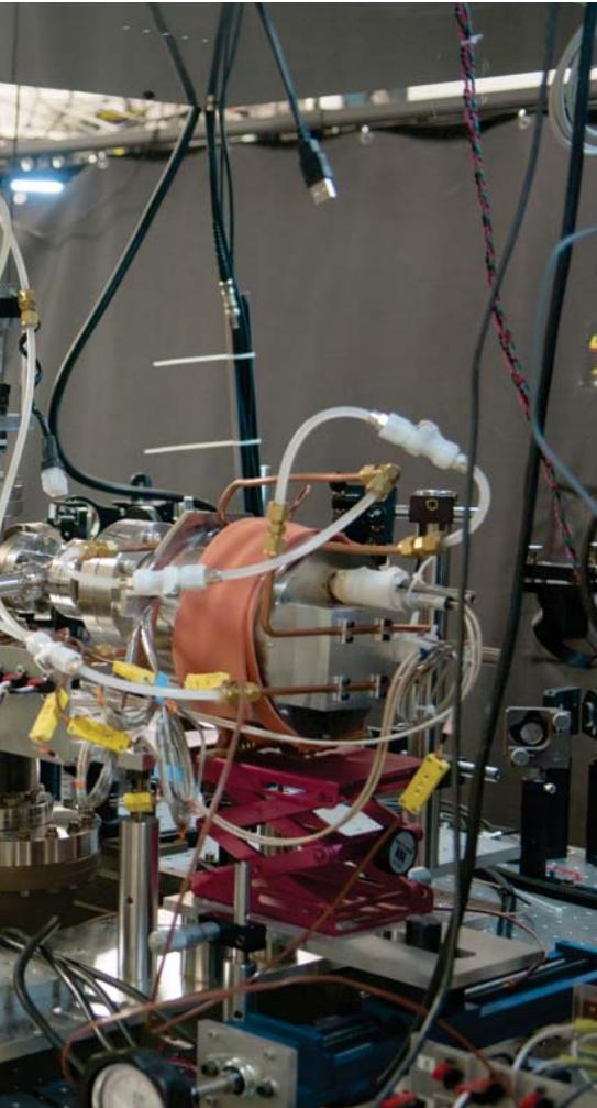
A new separator along the lines of a modern calutron at Oak Ridge National Laboratory will start producing small quantities of various stable isotopes this fall, and plans are in the works to increase production capability to kilograms.
