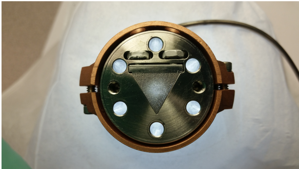
Figure 5.5: Image of the assembled nozzle of the directional oven. Within the triangular cutout are 2485 capillaries in a hexagonal packing arrangement and are fixed with a small clamp.
