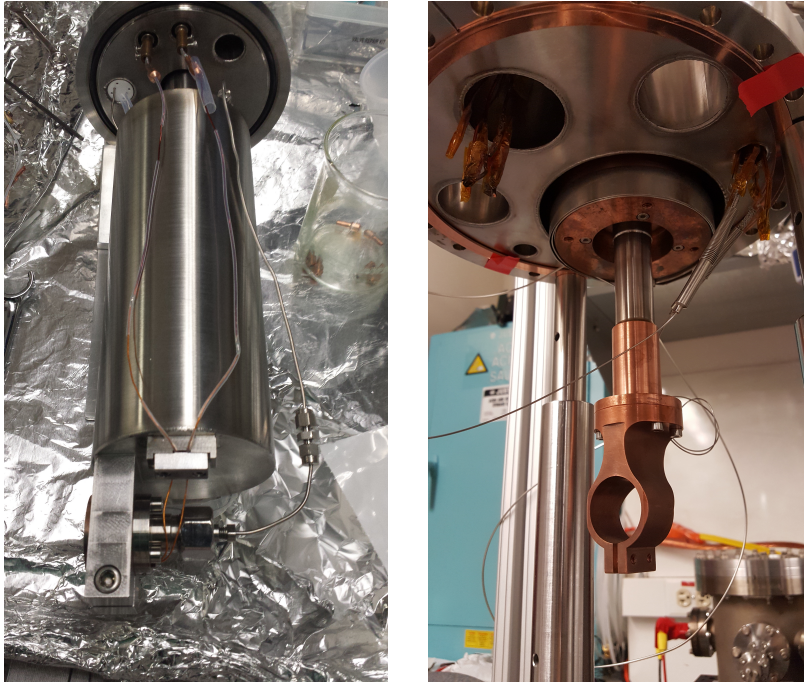
Figure 5.2: Cooling the supersonic nozzle with a liquid nitrogen dewar (left) and a helium cryocooler (right).
