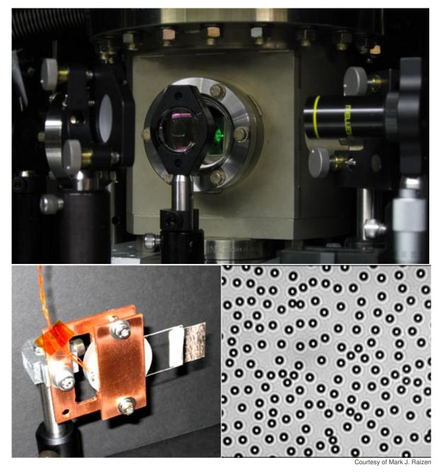
Raizen's team in Texas came up with a creative new experimental design, starting with a gas medium for their Brownian particle. Then, using a neat trick called "optical tweezers," Raizen and colleagues successfully captured instantaneous speeds of a tiny bead levitating in gas. ABOVE: The bead trapped
