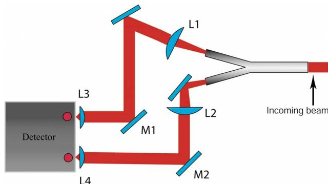
FIG. 1. (Color online) Schematic of the complete position-sensitive detector. The fiber optic waveguide splitter splits an incident beam into two equal parts. Lenses L1 and L2 serve to collimate the light. The light is directed with mirrors M1 and M2 and focused onto the balanced photodetector with lenses L3 and L4.
