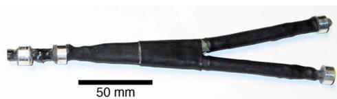
FIG. 4. (Color online) Photograph of completed split fiber bundle. The bundle is 8 in. in length and the two back ends are split about 2 in.
