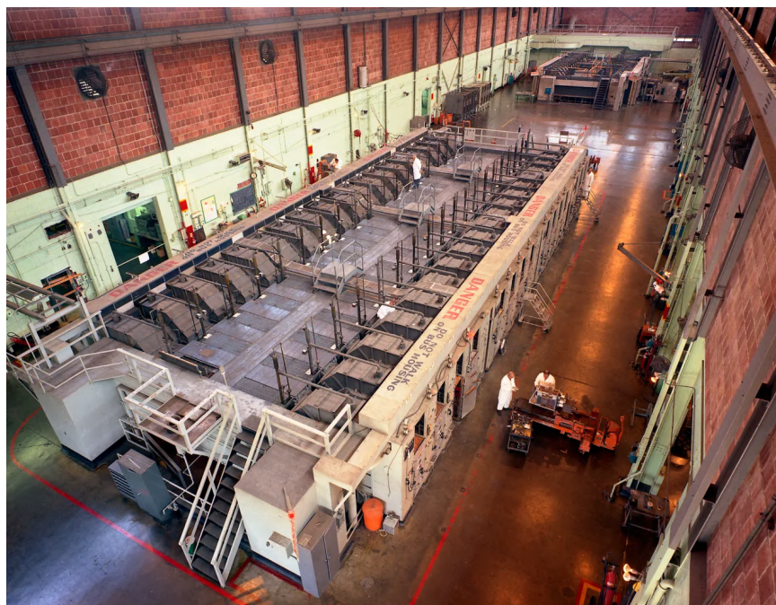
Figure 3.3: Calutrons used at ORNL for stable isotope separation through 1998 [281].
