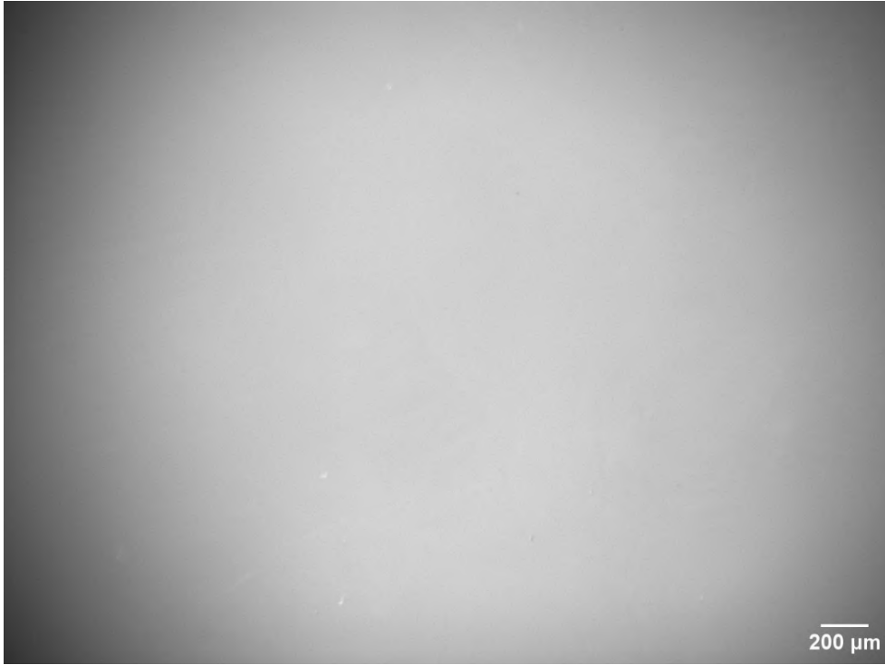
Figure 4.2: PDMS surface viewed under optical microscopy ( \sim 1\ \text{mm} \times 1\ \text{mm} ). The coating contains sparse micron-sized impurities or imperfections, separated by more than 0.5 - 1\ \text{mm} . [365]
