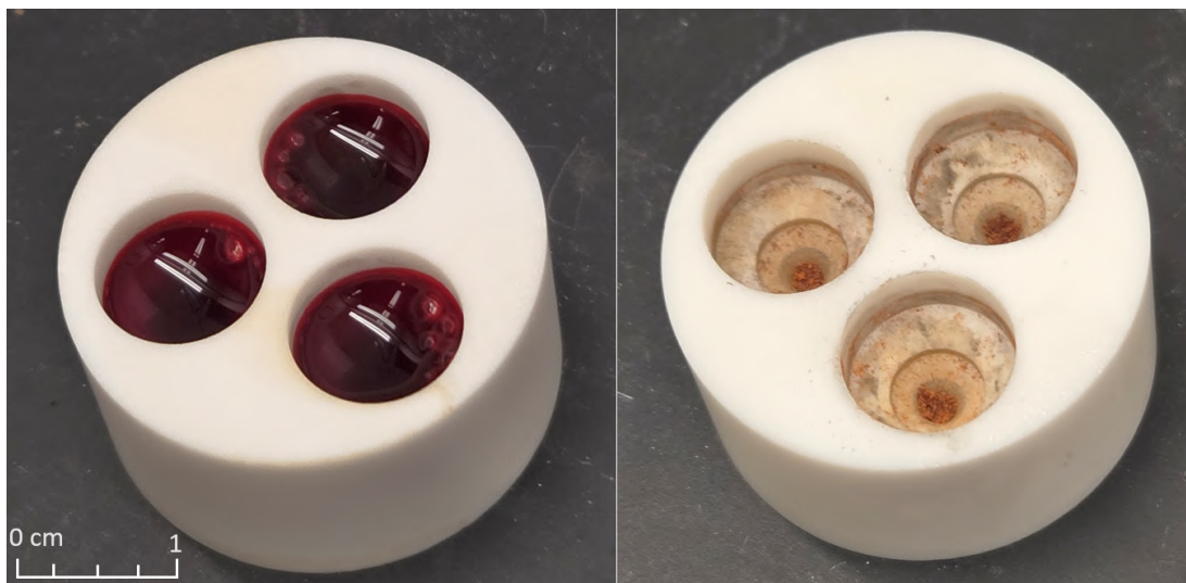
Figure 2.8: Left: 3 \times 150 \mu\text{L} whole blood samples. Right: samples after ashing.
