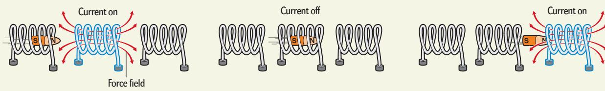
**1** Current in a coil generates magnetic forces that push a particle (bullet) away from the coil. An approaching particle thus slows down.
